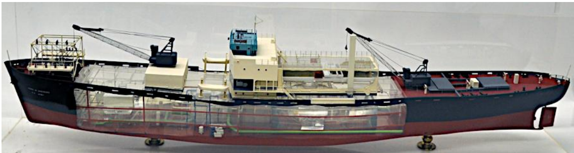
The reactor replaced the propulsion system of the USS Sturgis, converting it into a floating nuclear power plant (Army Engineer History)
