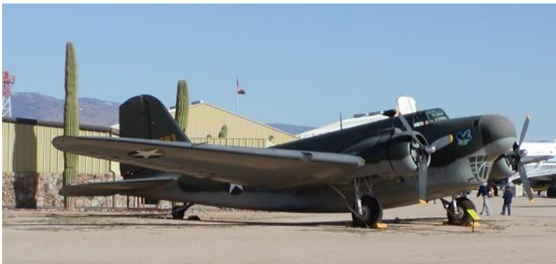
B-18B Bolo fitted with SCR-517 radar in a modified nose (Pima Air & Space Museum photo)
