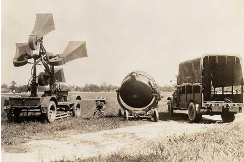
A mobile anti-aircraft “Big Ears” sound locator unit of the Coast Artillery Corps, with a searchlight, in 1932
