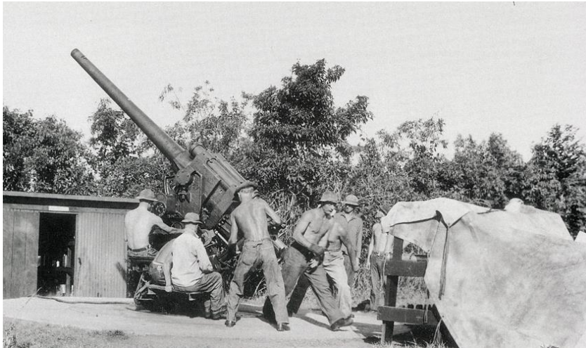
3-inch gun AA battery. The standard anti-aircraft gun would be upgraded from the M3 3-inch gun to the M1 90mm gun 11
